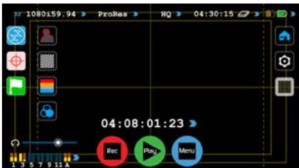
SAFE AREA/GRID LINES SHOWN WITH MENU OVERLAYS
